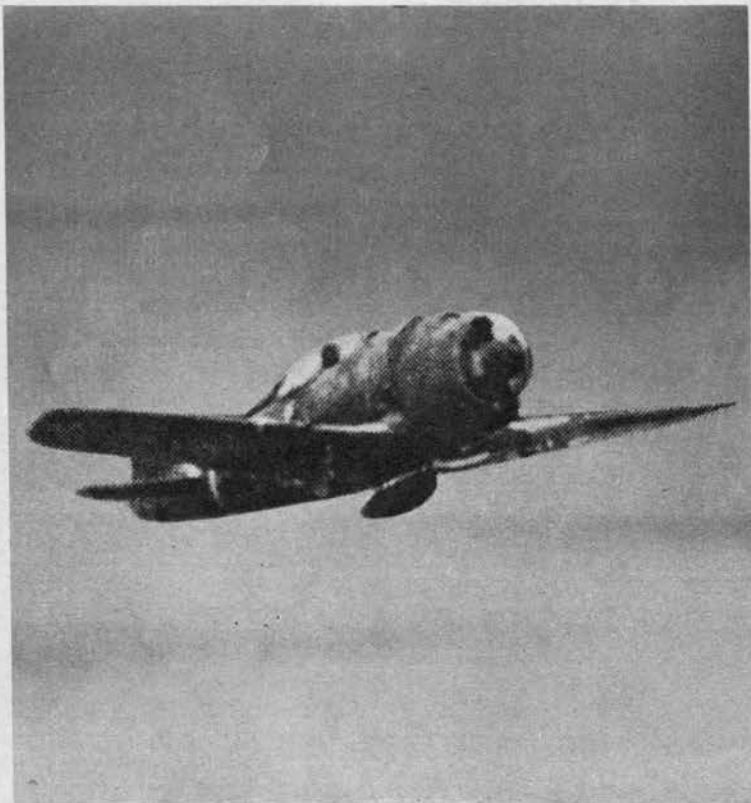
TOJO Somewhat chunky for a Japanese fighter with its barrel-shaped radial cowling, Tojo retains characteristic Jap fuselage which thins out sharply to a long stinger-like tailcone.
